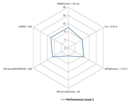
System parameters: Industrex scanner HPX-1 Plus S/N 1765 IP plates Flex HR type 6537 Scan resolution 25  $\mu m$  Laser low PMT sensitivity 100
